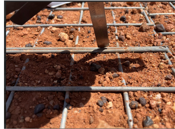
Example of using a feeler gauge to measure the separation distance of the slot. This is an example of a slot with a small distance separation <0.25\text{mm}
