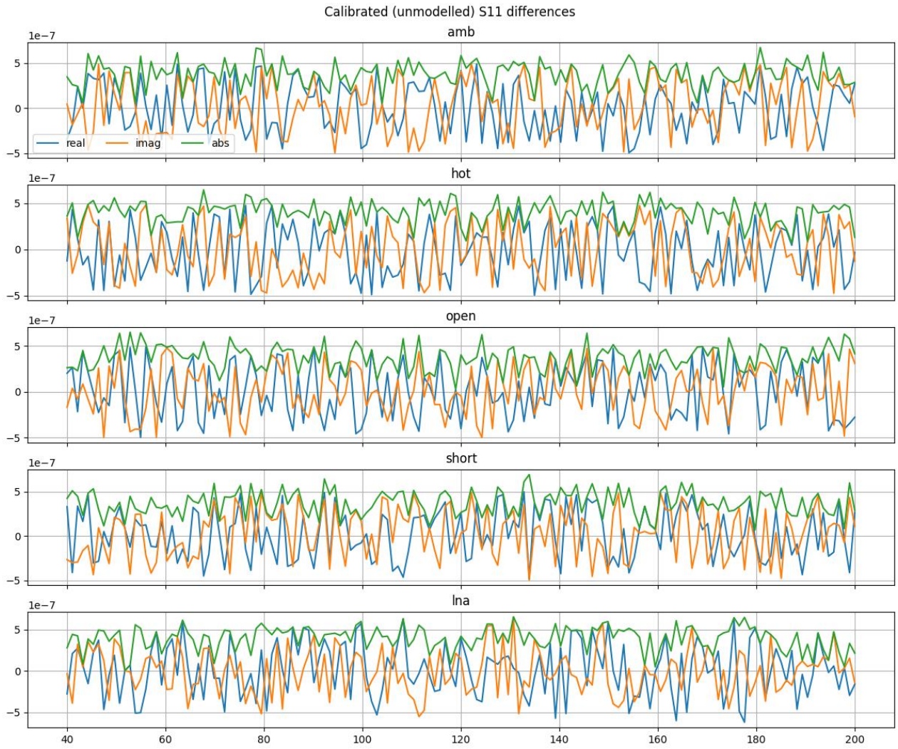
Figure 3: Difference in unmodeled S11 obtained from Alan's pipeline and edges-cal.
