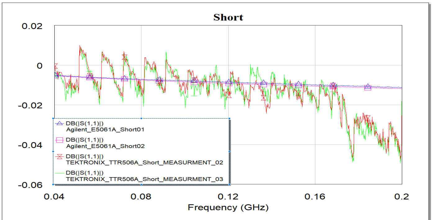
Figure4: Magnitude of the Short after calibration. Tektronix TTR506A measurement one red trace, Tektronix TTR506A measurement two green trace, Agilent measurement one blue trace, and Agilent measurement two pink trace. The difference in noise between the two VNAs with the same settings is favoring the Agilent E5061A VNA due to consistent curvature.
