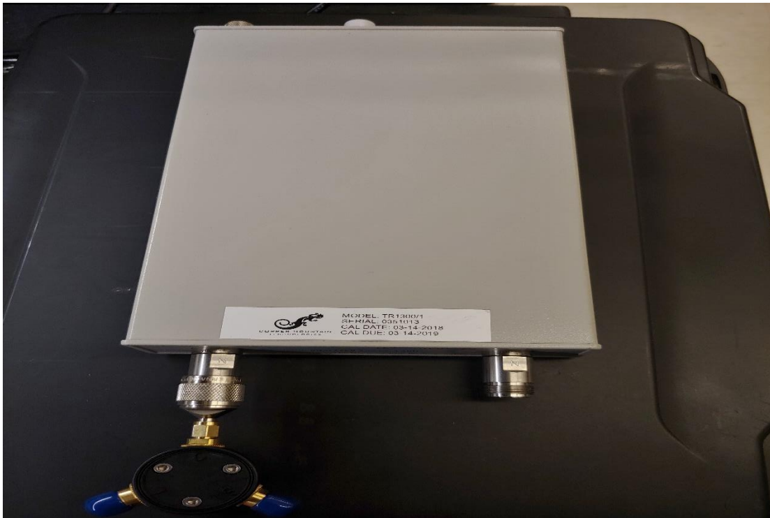
Figure2: Copper Mountain TR1300/1 Calibration arrangement utilizing the male 85033E Calibration kit
