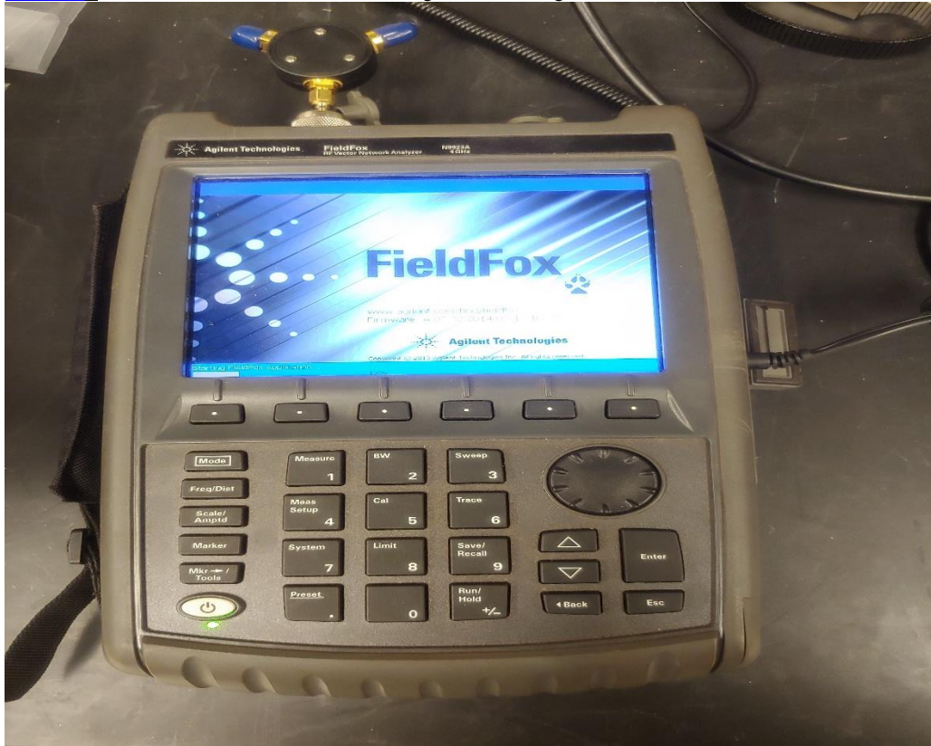
Figure2: AGILENT FIELDFOX N9923A Calibration arrangement. utilizing the male 85033E Calibration kit
