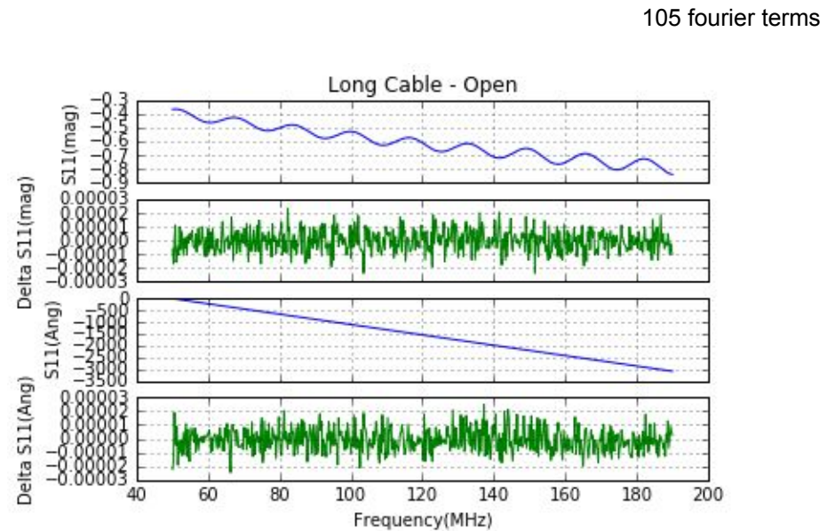
Figure3b: Reflection coefficients of the long cables. Blue is the fit to the S11s (mag & phase). Green is the difference between the fits and the actual measurements for each respective case.
