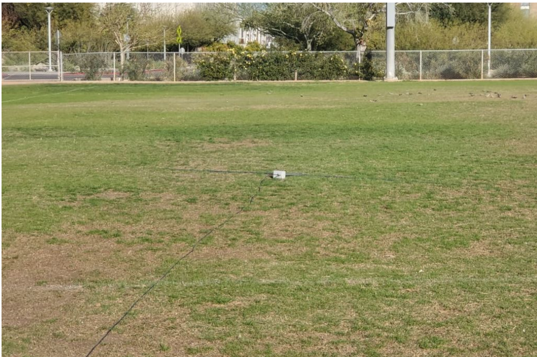
Figure1: Measurement set up of the dipole on the ground at the SDFC field. The other end of the coax is connected to a VNA.
