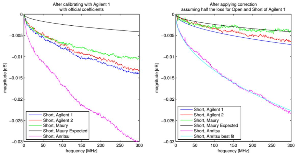
**Figure:** (1) Comparison of measurements, corrections, and expectations of four *short* standards belonging to different calibration kits. The previous slide provides more details.
