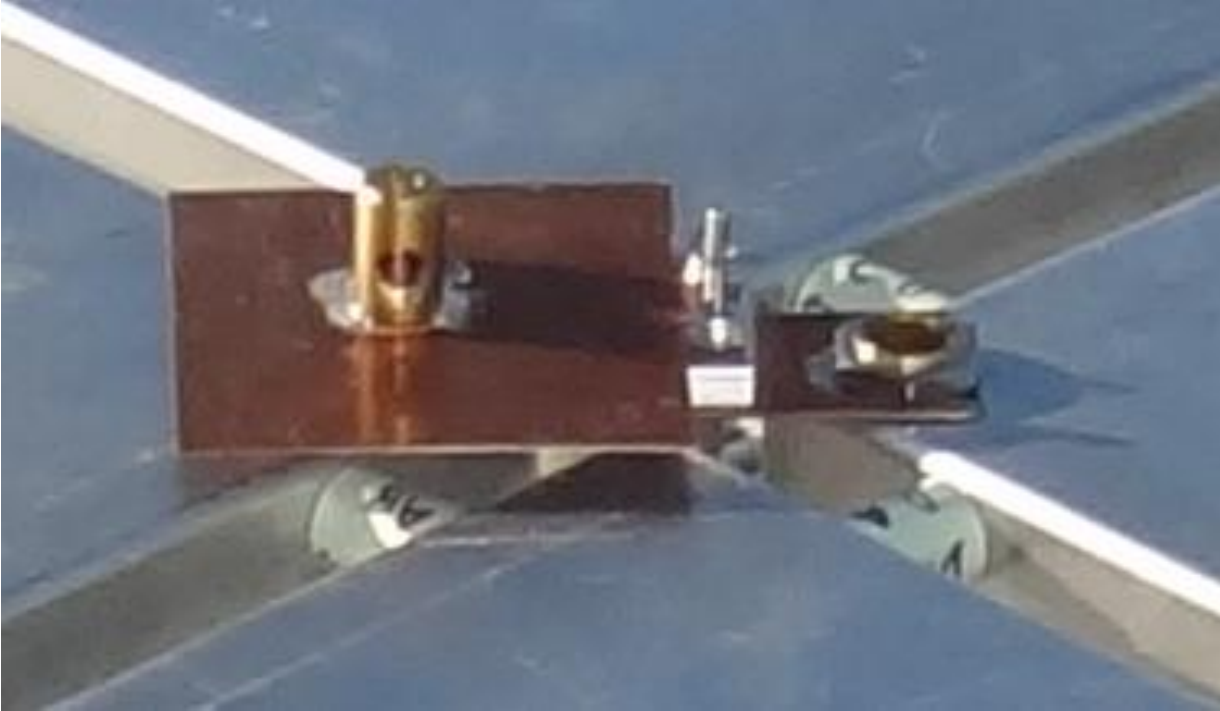
Figure 1. Top plate capacitor. Stub connection on the right open tube balun.
