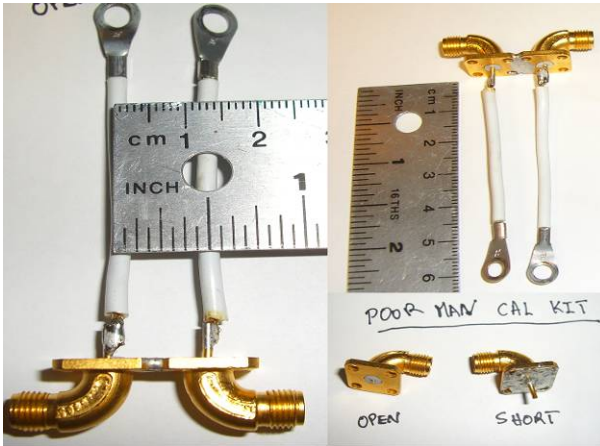
Fig2. TL used for the impedance measurements. Also the home made cal kit used to remove the effect of the SMA connector.
