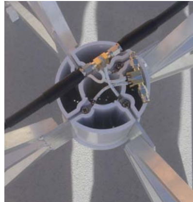
Fig20. Top: the VNA was placed as far as cable length allows from the antenna. Bottom: connection to one polarization of the antenna while the second polarization is terminated in 100 Ohm (2X50 ohm terminations)
