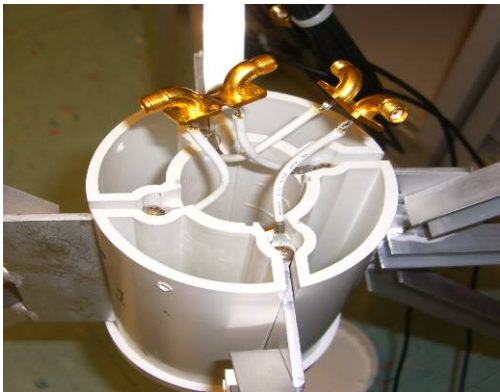
Fig3. The 2 polarizations of the antenna with SMA connectors ready to be measured.
