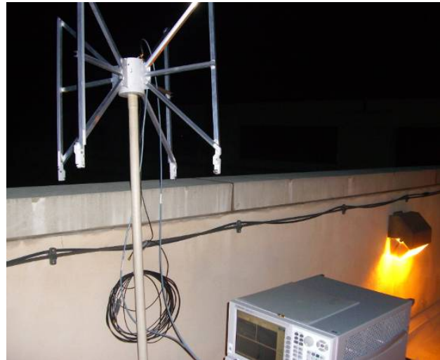
Fig4. Measurement setup on the west side of Caltech's Moore building showing the antenna far away from any wall or conductive objects.
