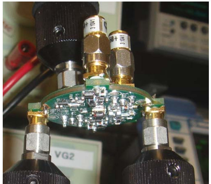
Fig1. MWA Dual LNA with SMA connectors soldered to the input and connected to the VNA. All ports not connected to the VNA are terminated with 50 Ohm load.
