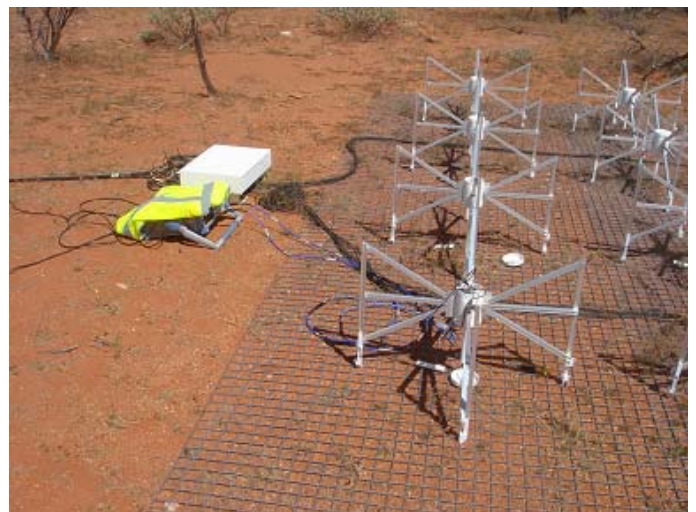
Fig15. Measurement setup showing the antenna, cabling and the VNA.
