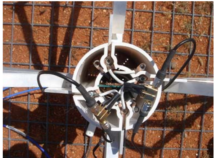
Fig14. Connection to the antenna during polarizations coupling measurement.
