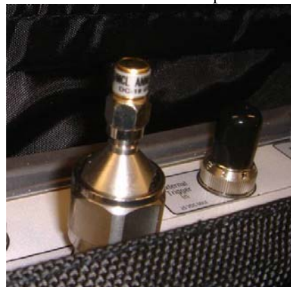
Fig1. the measurement setup showing a mini circuits termination connected to port1 through a type-N to SMA adapter.
