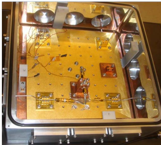
Fig. The cryostat used to cool a termination to 9K. This setup was used to compare the solid state noise source and the thermal noise source. The setup was used also to compare the smoothness of the output spectrum of the noise source compared to 300K and 9K thermal noise sources.
